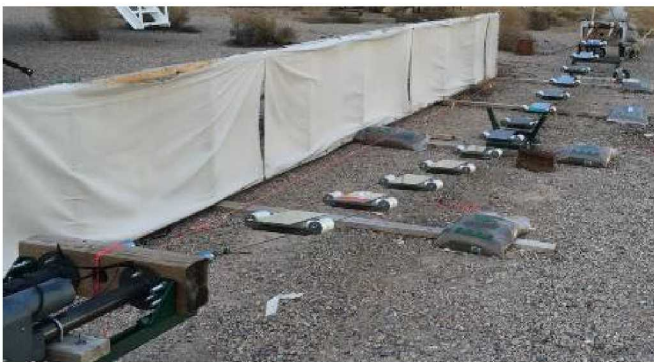
FIGURE 4. Image of Prototype 3 set-up with another wind fence on the east side. The wind fence impacts were studied as part of the mechanical evaluation [36].
