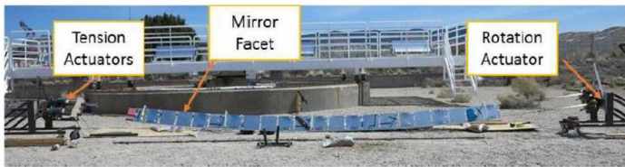
FIGURE 1. Image of small-scale Prototype 1 system. The horizontal distance over the cable span was about 9.1 m. The flat-plate receiver is located about 12 m to the right (not seen in the picture).
