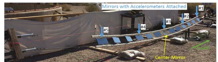
FIGURE 8. Prototype 2 set up with accelerometers attached to the five mirrors. In the Prototype 3 set up the same mirrors had accelerometers attached to them.
