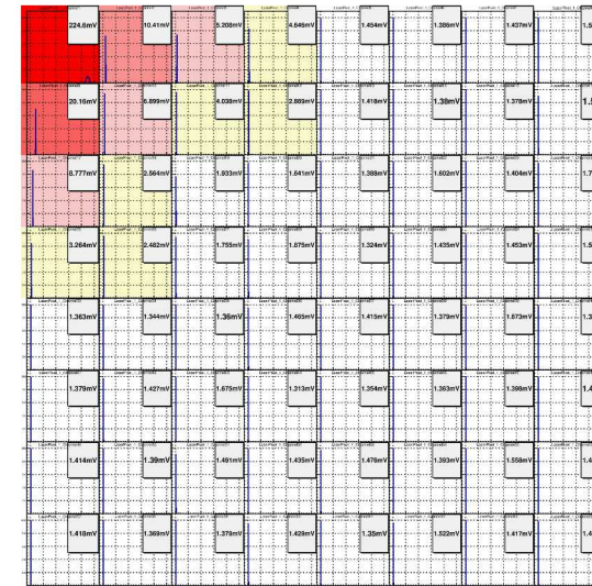
Crosstalk correlation among the SiPM pixels, the red pixel corresponds to the channel illuminated by a laser, the color represents the amplitude of the crosstalk.
