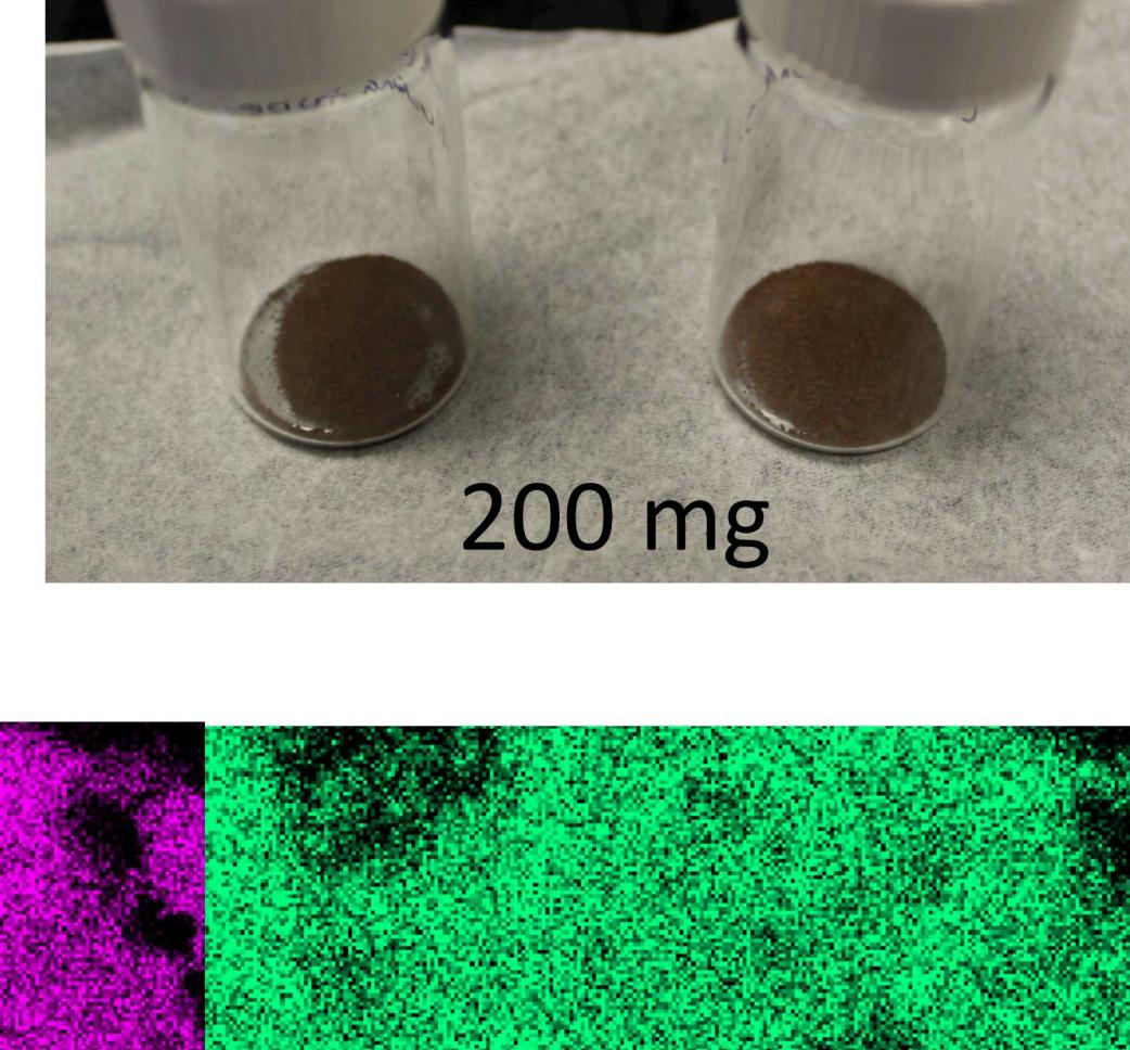
Particles form by supersaturation and nucleation as spray droplets evaporate. Fluid flow rate, controlled by gas pressure, dictates synthetic yield per unit time. Product exhibited requisite single-phase crystallinity and co-location of all precursor elements. Median diameter is 128 nm
