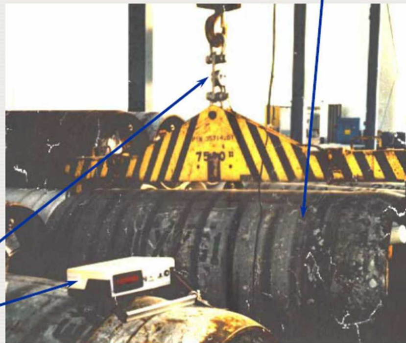
Load cell being used to weigh a UF 6 cylinder
