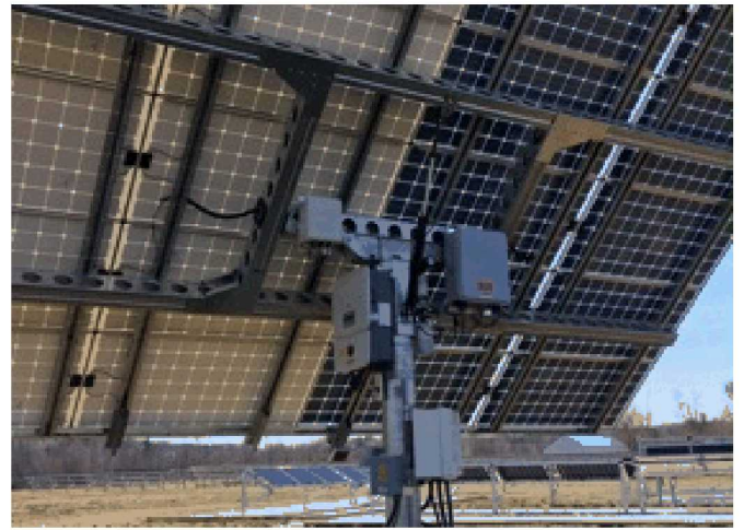
Fig. 16. Backside of Tracker One, with DC monitoring box and datalogger mounted on the pedestal. Monofacial modules are on the left side; bifacials on the right. Backside shading proved to have minimal impact on the bifacial gain for this system.
