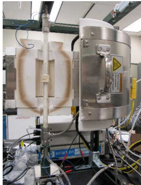
Top: assembly of membrane cell
