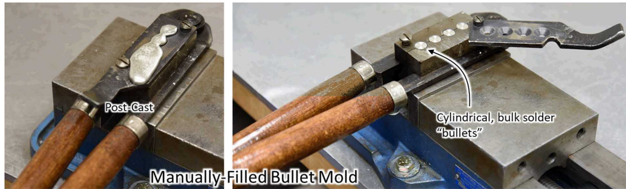
Figure 2. Bullet mold immediately after molten solder was poured (left) and after rotating the mold top (right).
