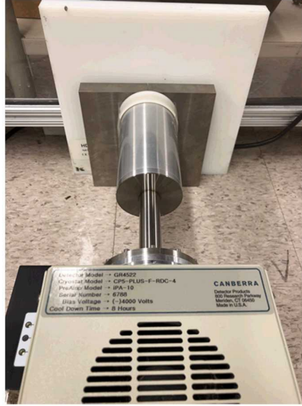
Figure 9 – Photograph of measurements made of the tungsten shielding. After neutron exposure, the shielding was placed on the floor approximately 6 feet from the H-Gear and measurements were made with the face of the detector in close proximity to the outer surface of the shielding.
