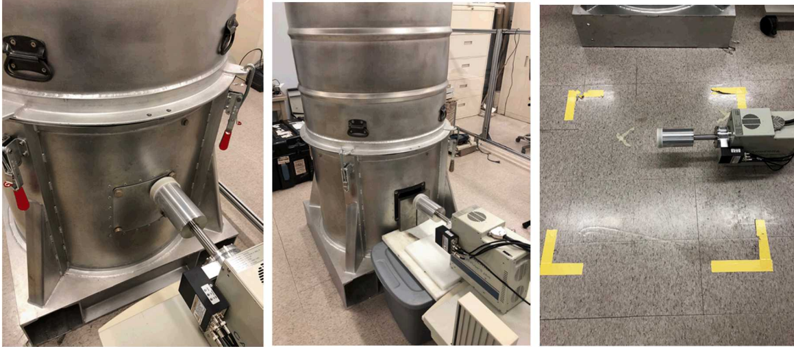
Figure 2 – Photographs of the H-Gear and the HPGe detector set up with (center) and without (left) a tungsten shield and measurements on the floor underneath the H-Gear (right). The yellow tape marks indicate the position of the H-Gear during neutron exposure.
