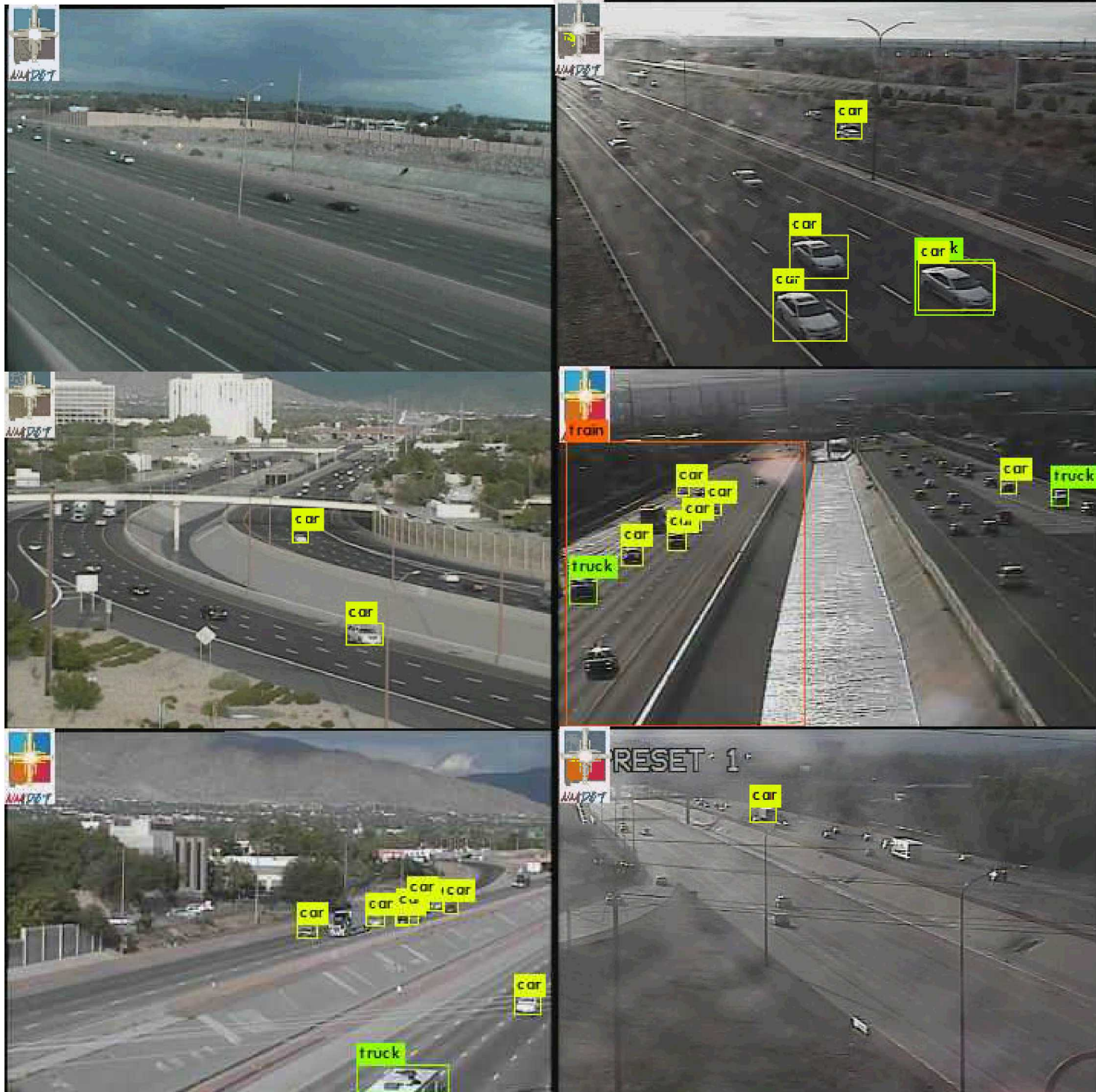
(Above) ML algorithm applied to NMDOT camera's of the I-40, 7/14/19 at 7:20pm (top left) at University, (top right) at Carlisle, (middle left) at San Mateo, (middle right) at Louisiana, (bottom left) at Pennsylvania (bottom right) at Eubank
