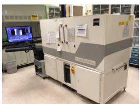
Using a 3D Systems Pro X DMP 200, an “L-column” geometry was printed from 316L stainless steel powder having intentional 1) internal cavities of prescribed size and 2) intermittent porosity throughout. Laser power was fixed at 103W, with a beam diameter of 100 $\mu\text{m}$ , a nominal powder layer of 30 $\mu\text{m}$ , hatch spacing of 50 $\mu\text{m}$ , and a build velocity of 1.4 m/s.
