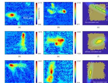
Temperature estimates for normal and outlier melt pools are shown above in the left and middle columns. The corresponding best fit ellipses for each are presented in the right column overlaid atop corresponding micro-CT layers.
