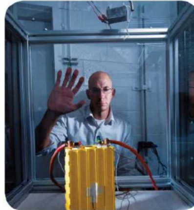
A Sandia researcher prepares to test a battery to determine its response under abuse conditions.
