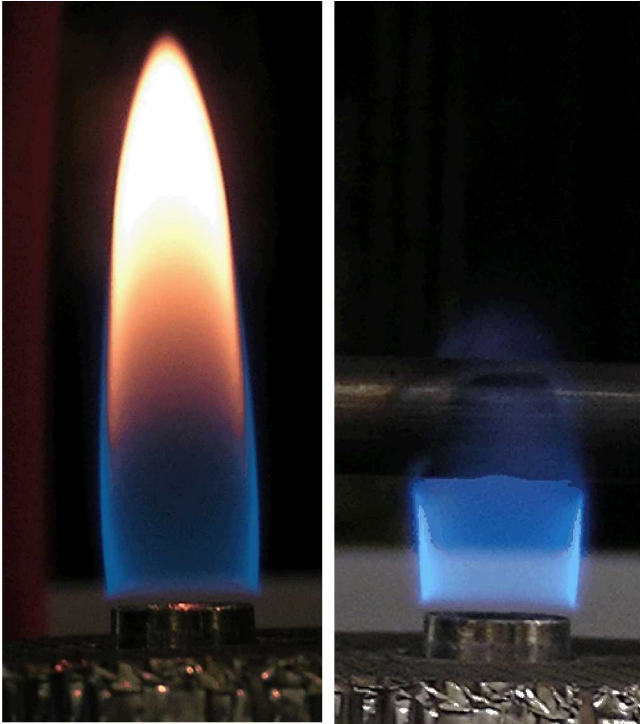
Co-flow diffusion flame
