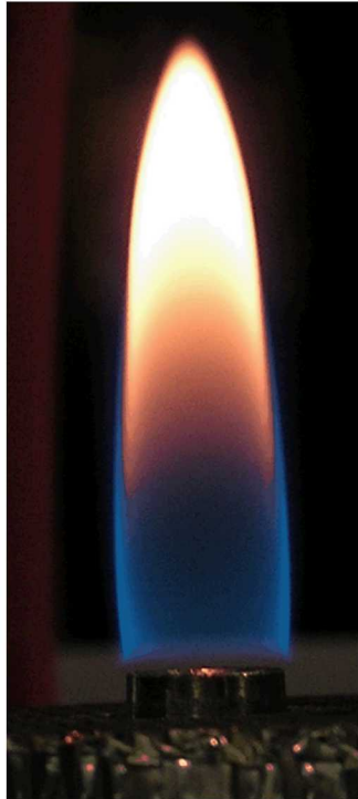
Co-flow diffusion flame
