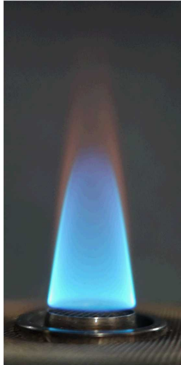
Partially premixed diffusion flame
