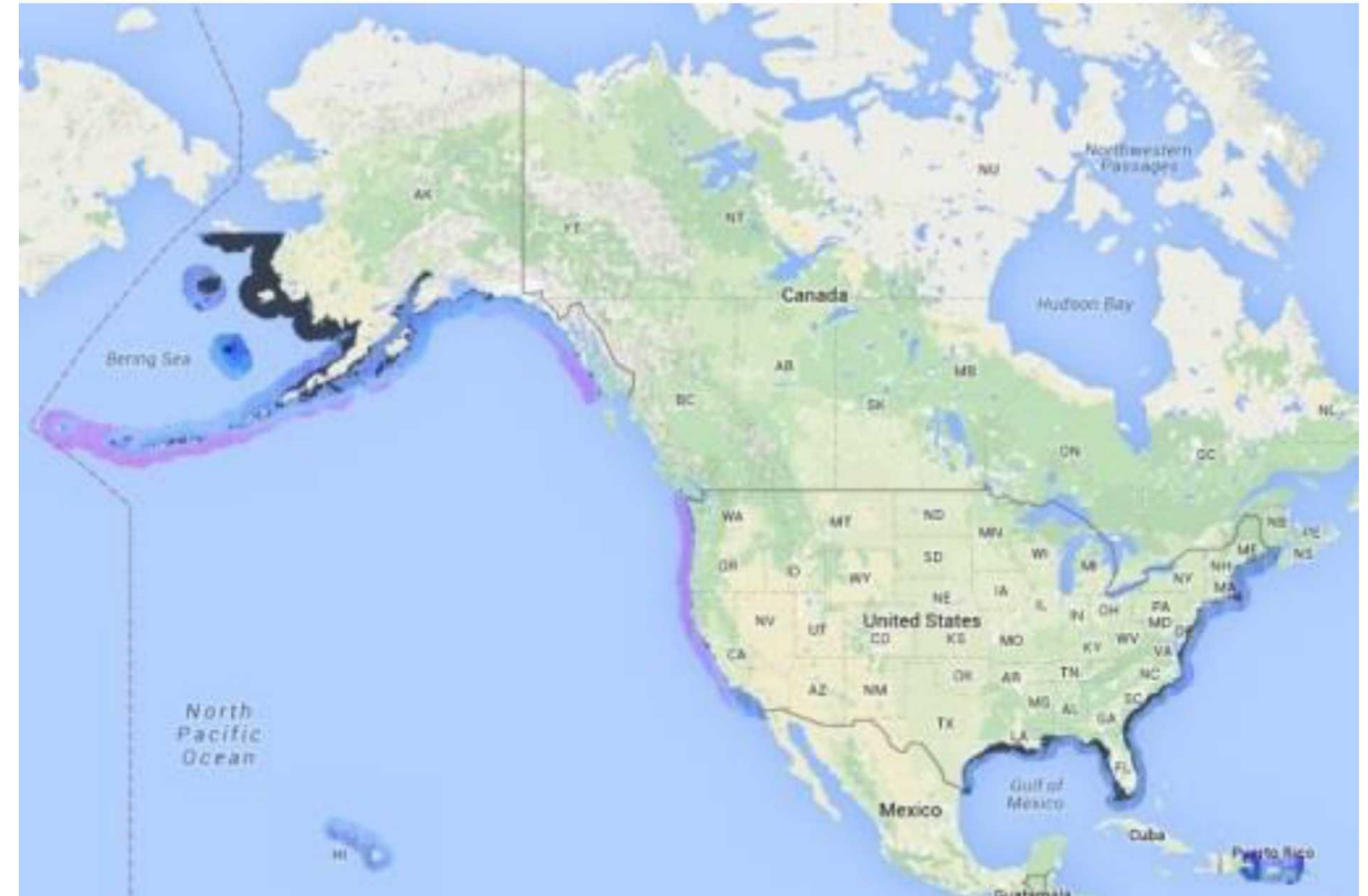
MHK Atlas showing spatial distribution of average annual omni-directional power density computed From NOAA WWIII 30-y hindcast [NREL 2019]
