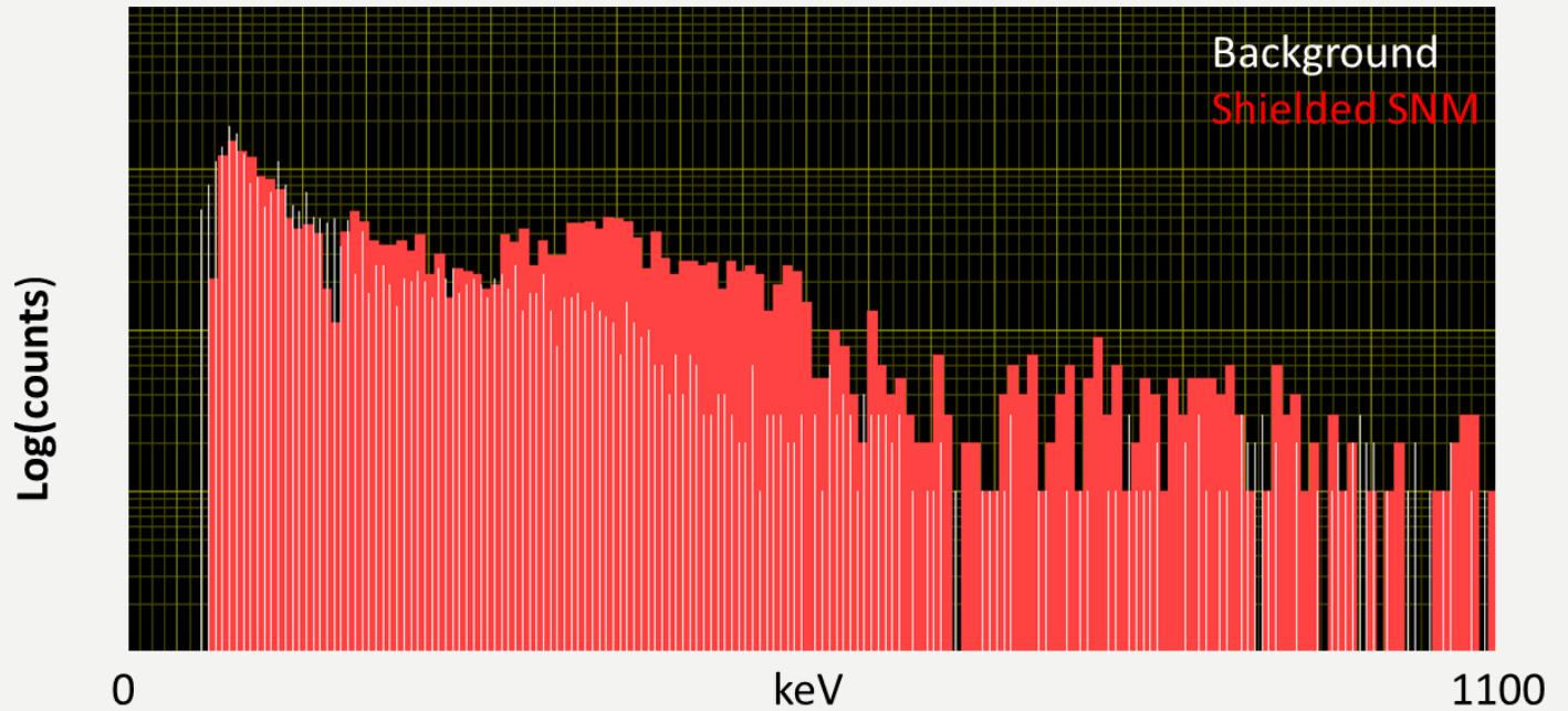
The red histogram (more events) shows results from a polymer-shielded small amount of SNM as a target. The white histogram shows a no target background. The difference between the two sets of results is clearest in the gamma energy range of approximately 300 keV to 500 keV.
