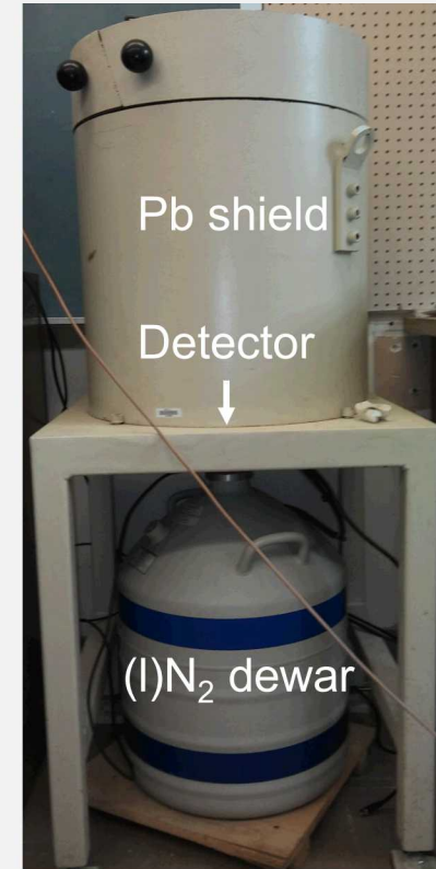
Fig 7. Ge(Li) gamma detector system with Pb shielding setup.
