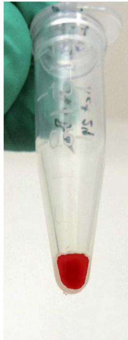
Photo of human whole blood stabilized in a AqS-based gel monolith
