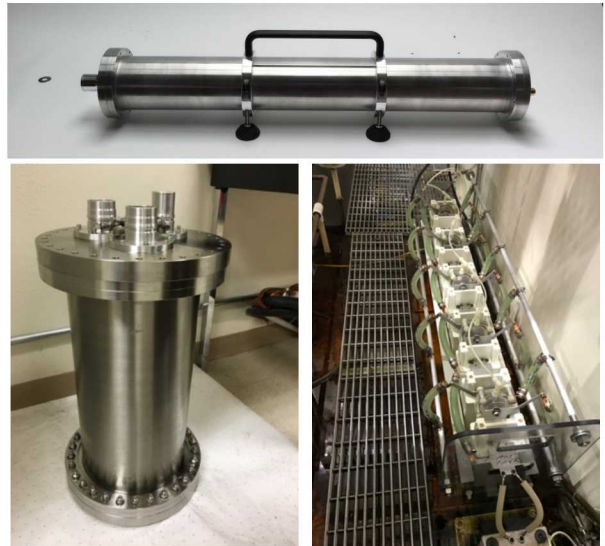
Figure 3. The APELC Marx bank (top) [6], the oil-filled cable junction enclosure (lower left), and the new MTG in the west oil tank (lower right).
