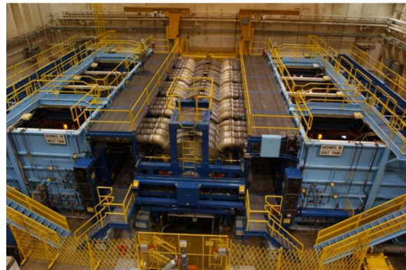
Figure 1. The Marx oil tanks (left, right) and induction cavities (center) of the HERMES III accelerator.
