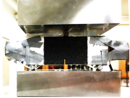
Fig. 3. Experimental setup: 3PB sample with top and bottom rods, acoustic transducers attached, and a speckled region on front surface for DIC.
