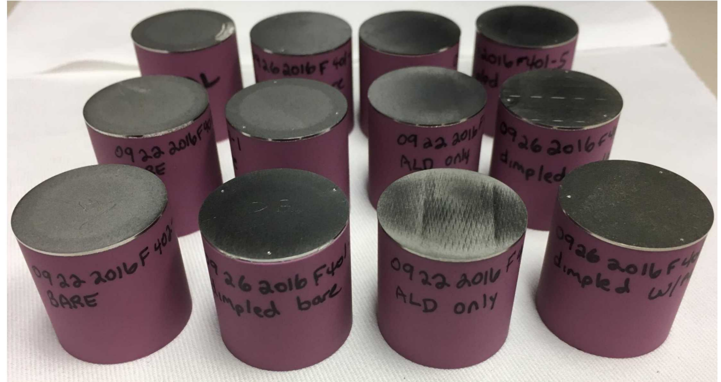
Active-brazed Diamonite cylinders to flush-mount Kovar flanges
