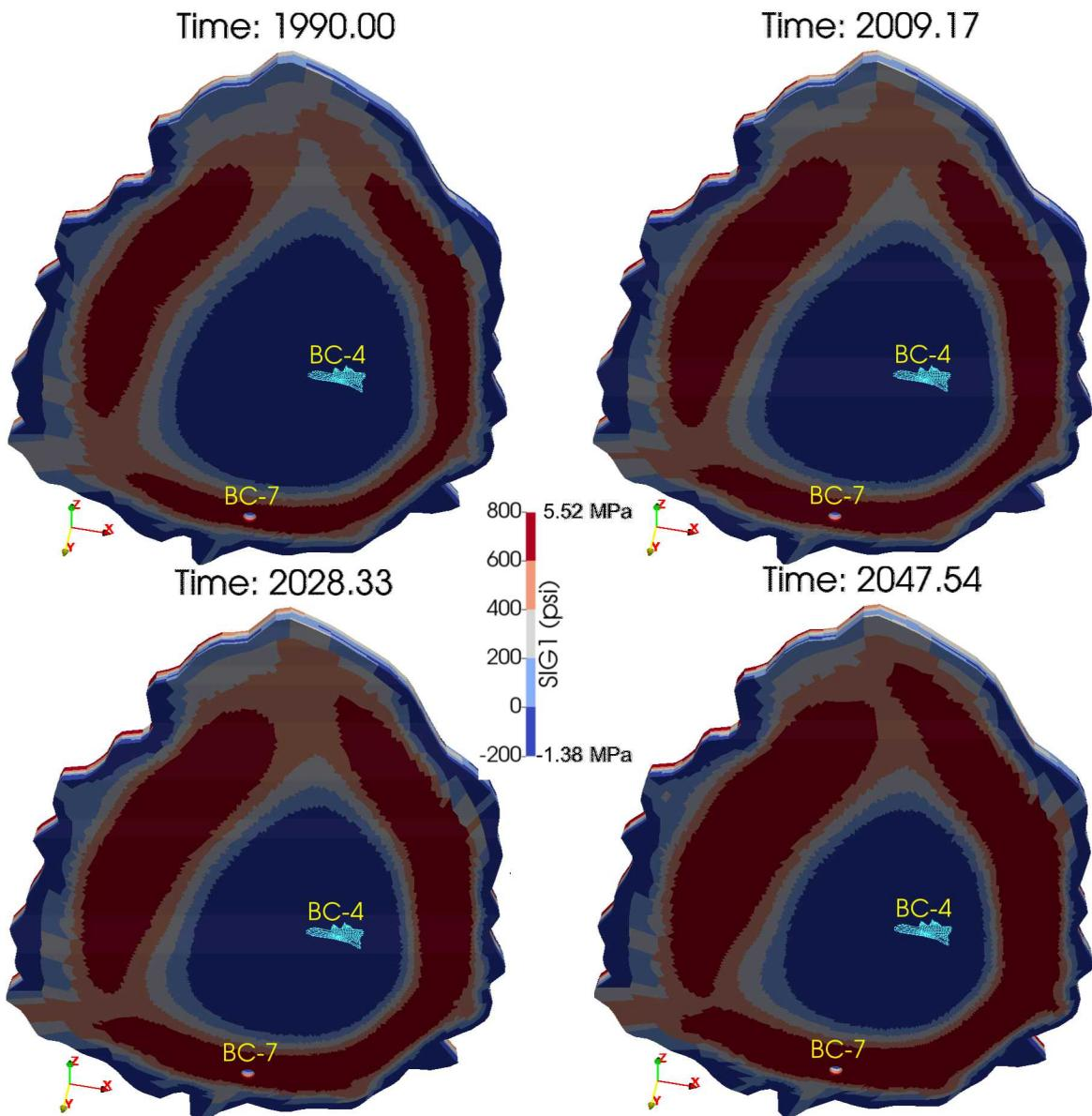
Contour plots of  $\sigma_1$  on the base of the caprock predicted for 1990, 2009, 2028, and 2047
