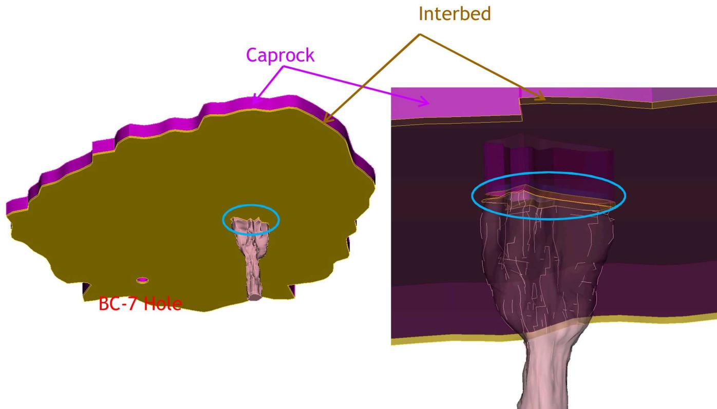
BC-4 is leached through three lithological layers, i.e. the caprock, interbed and salt layers
