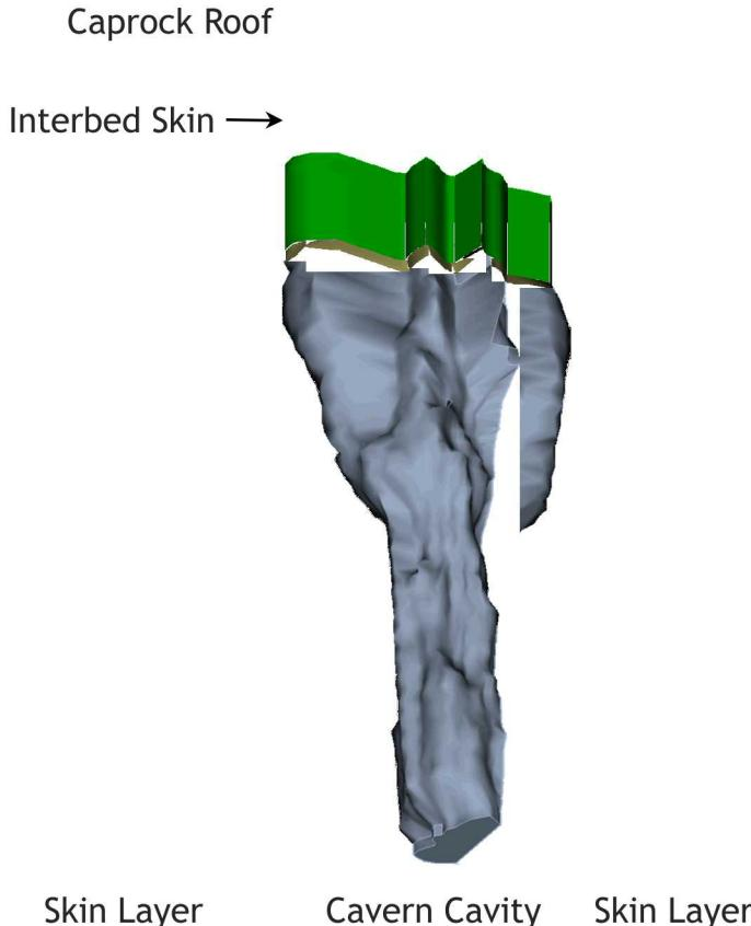
BC-4 cavern cavity with caprock roof along with a surrounding interbed skin and salt skin layer used in the geomechanical model
