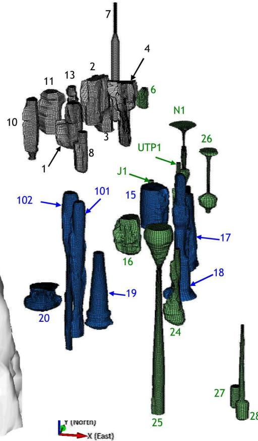
3D salt dome and caverns images based on the seismic and sonar survey data
