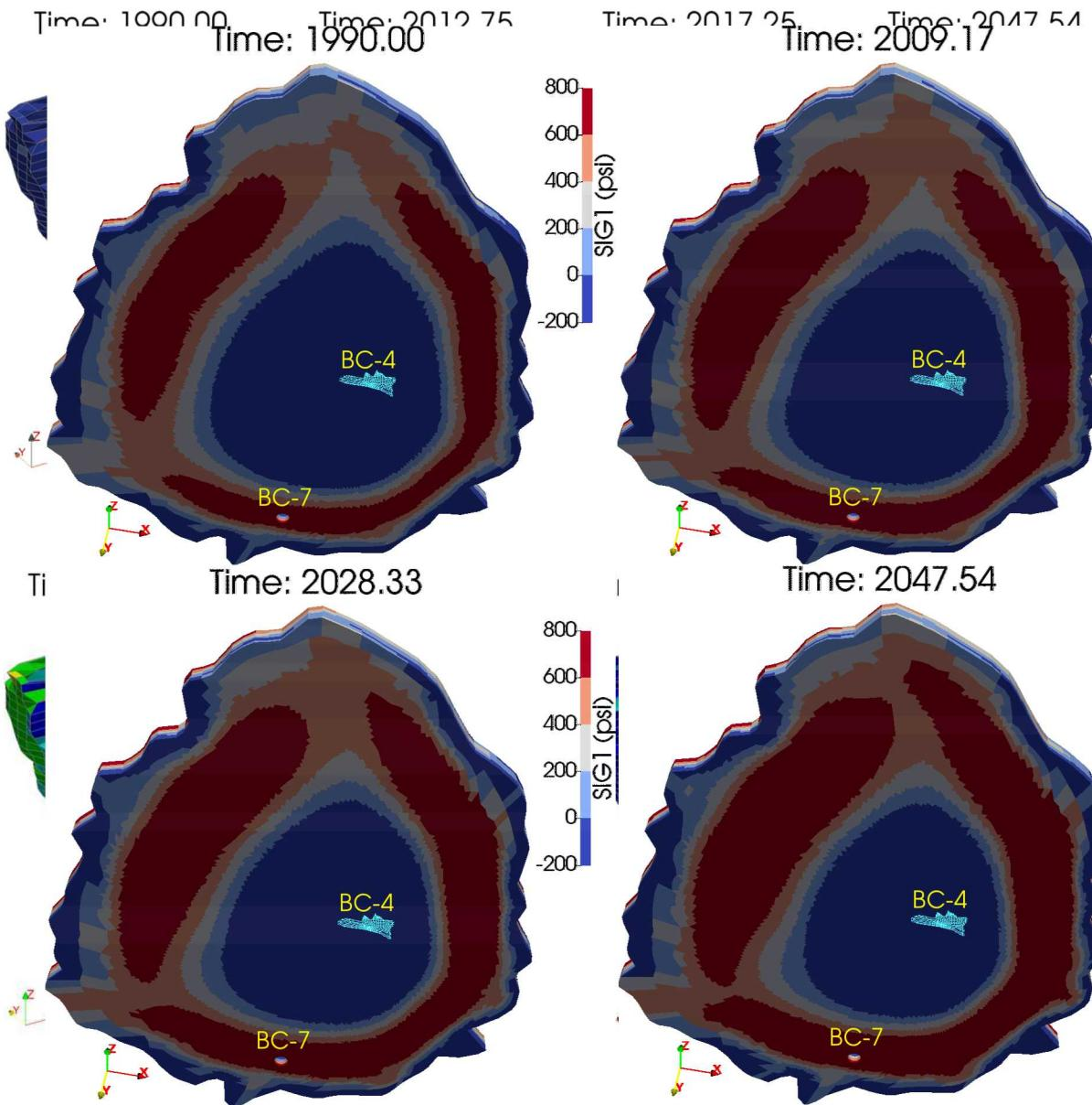
Cavern roof in the caprock layer has no predicted risk of structural stability in the form of tensile failure for up to 30 years
