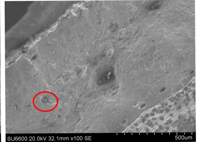
Unmelted particles on fracture surface
