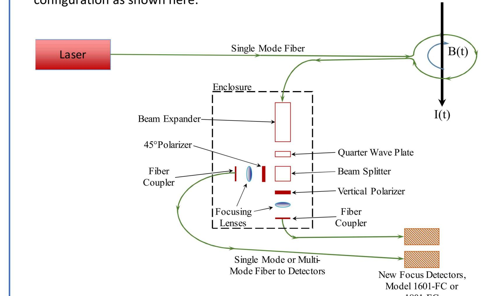
We purchased four sets of systems to include the laser, beam splitter assembly and enclosure and a pair of photo-detectors for each operating wavelength of 450nm, 520nm, 635nm, and 850nm.
