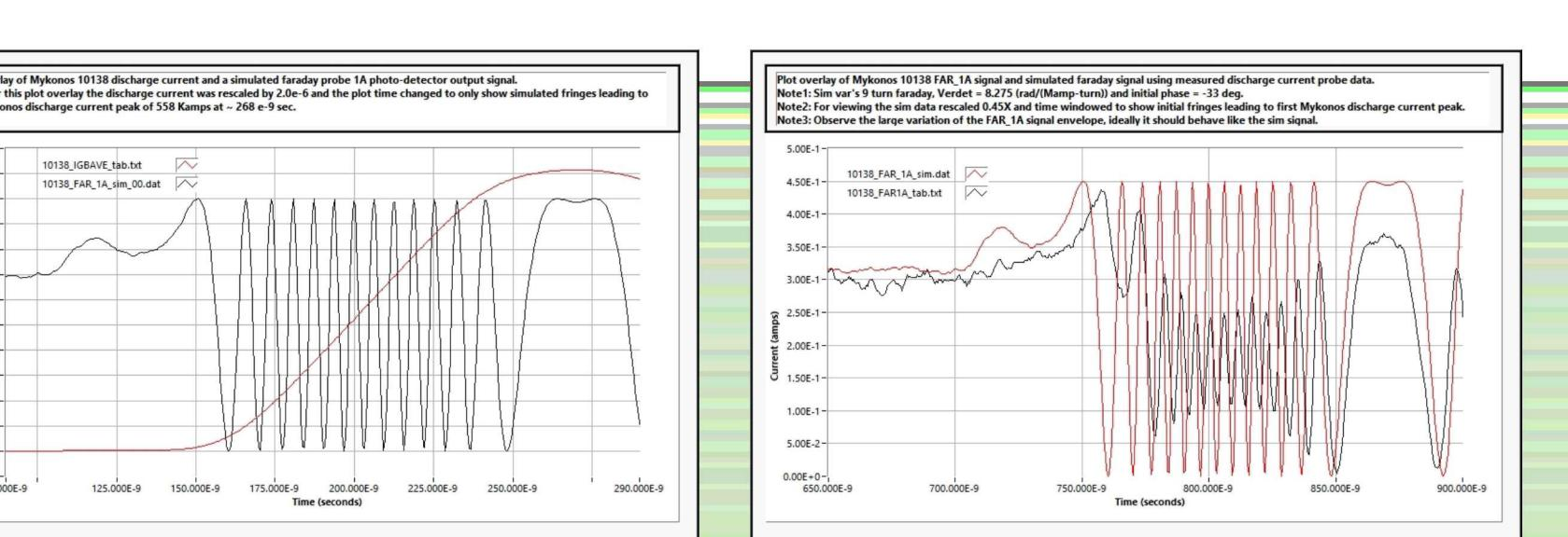
Notice that the plot on the left (simulated photo-detector) has signal fringe maximum and minimum that are uniform over the time window but the plot on the right (Mykonos probe "10138\_FAR\_1A") shows signal maximum and minimum that are varying throughout the plot window. This is indicative of a problematic probe monitoring system.
