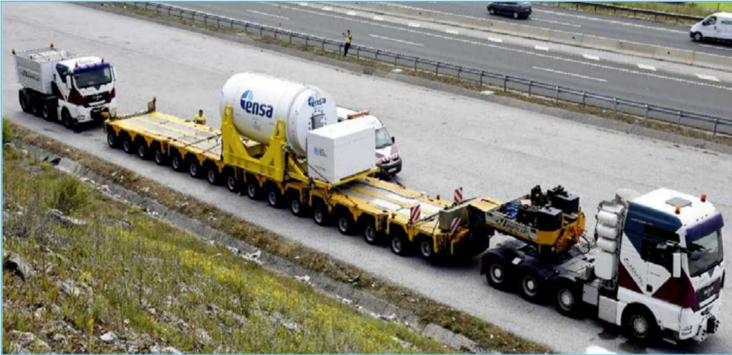
16-axle heavy haul truck transport through Spain
