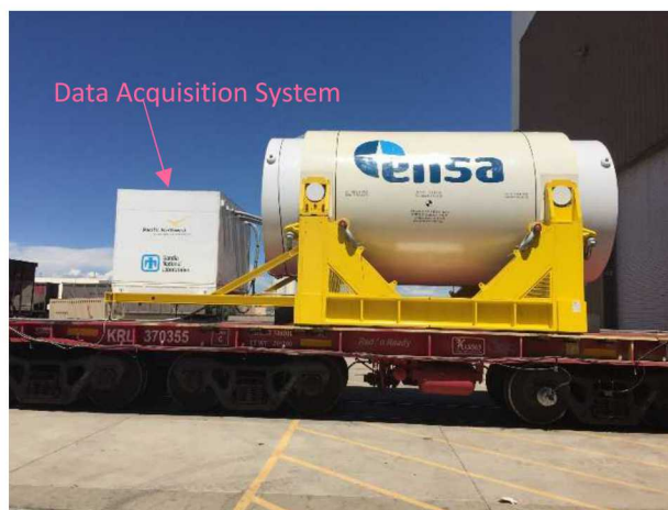
Figure 1. ENUN 32P cask on Kasgro 12-axle railcar used in rail transport.
