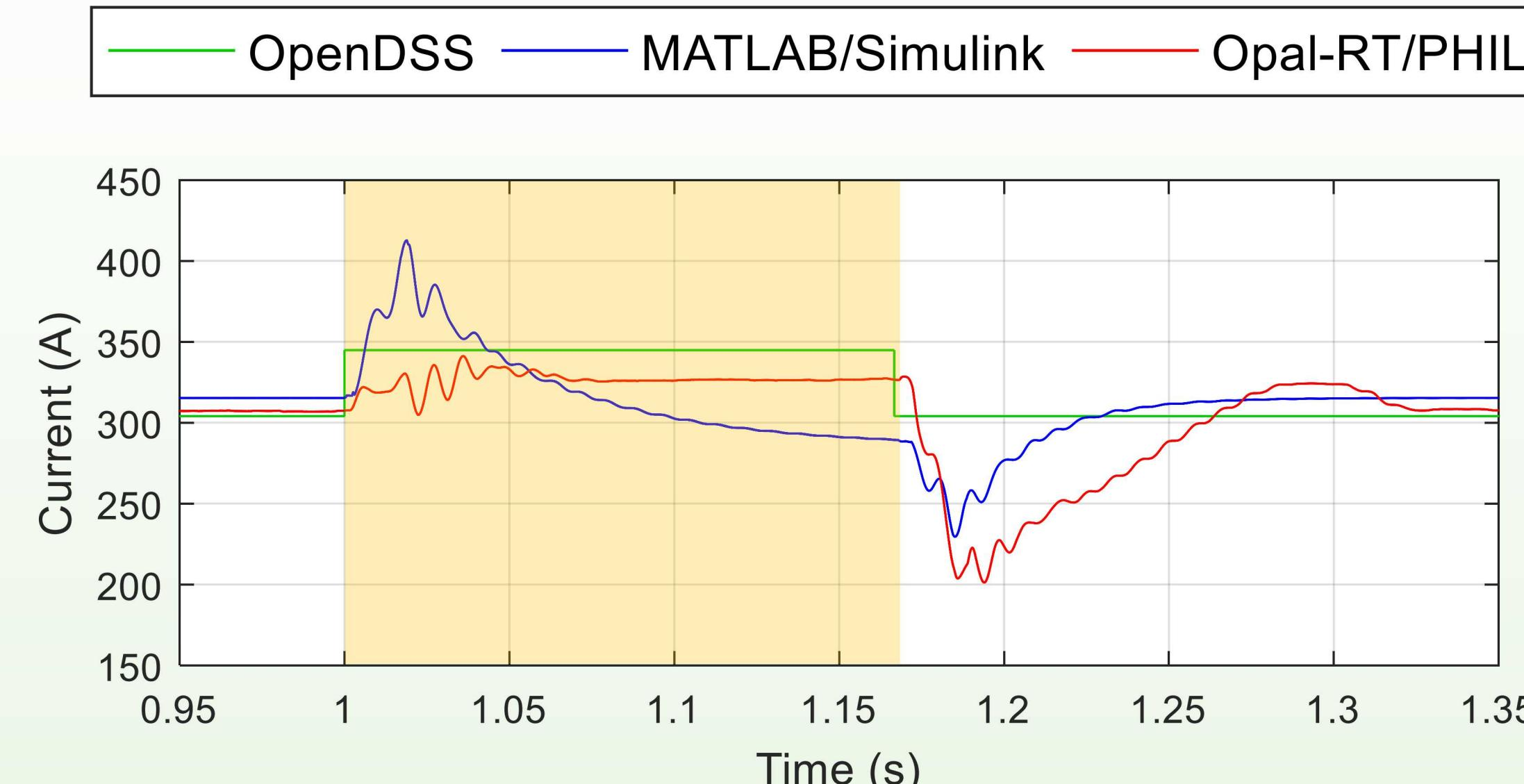
Introducing a 3-phase Fault at Bus 4, showed that all methods were closely correlated in steady-state, but the transient response of the inverter was difficult to capture with a PV model and the physical device behavior could not be represented completely without incorporating it through *PHIL/Opal-RT*.
