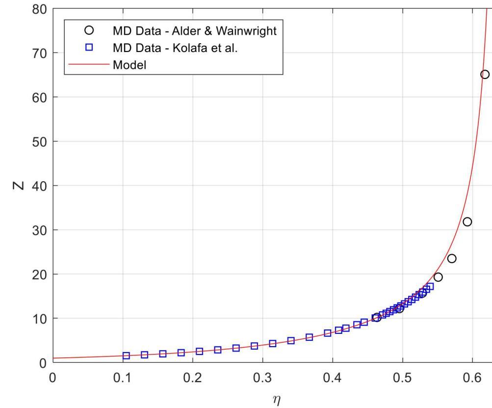
$$\Ζ = \frac{PV}{NkT} = 4\eta g_0(1, \eta) + 1 = 1 + \frac{3\eta}{(\eta_c - \eta)} + \sum_{k=1}^4 k A_k \left(\frac{\eta}{\eta_c}\right)^k$$
