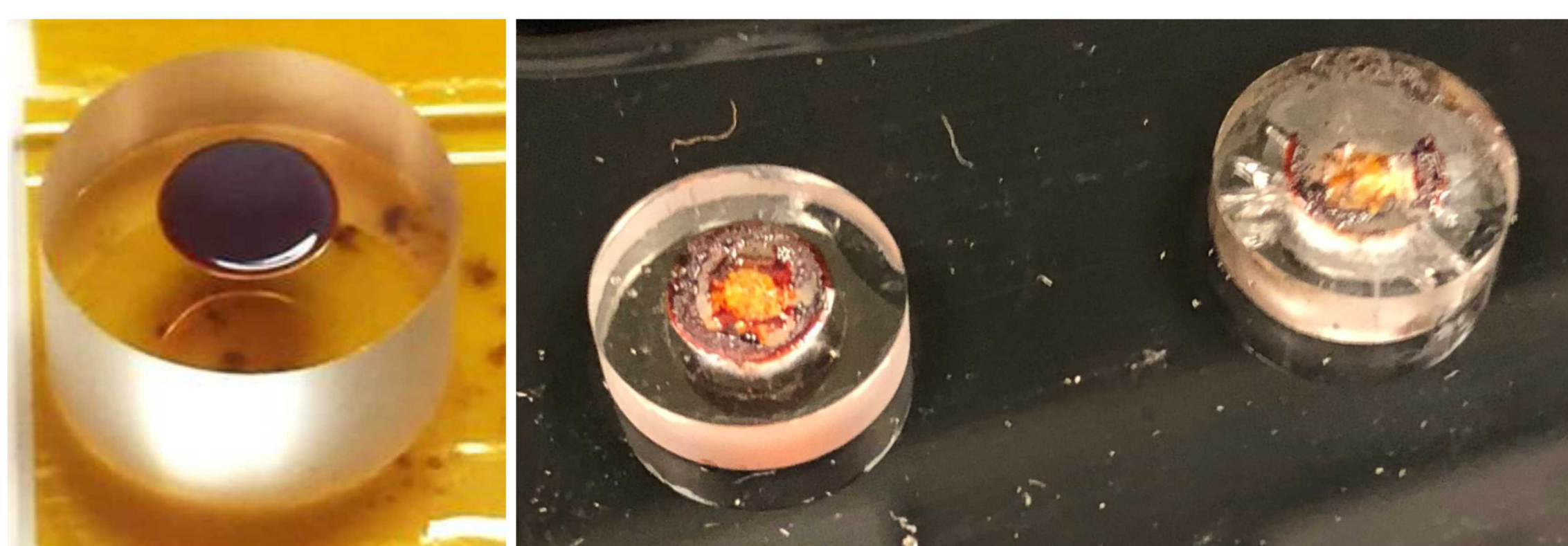
Left: Vapor deposited A-HNAB. Right: Shocked A-HNAB samples via flyer plate experiments illustrating shock induced crystallization.
