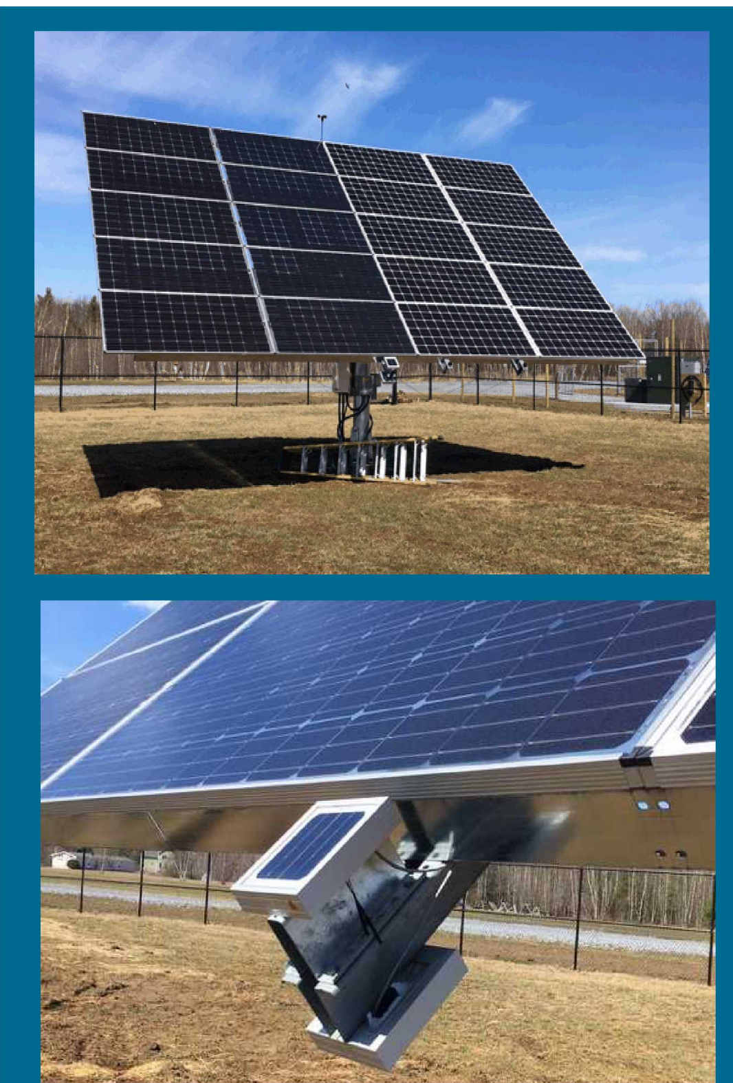
Figure 1. Bifacial dual-axis Tracker System Two. 72-cell bifacial modules populate the left half; 72-cell monofacials are on the right. Back-to-back plane-of-array EETS reference cells on the lower edge of the module measure irradiance on both sides of the tracker platform (right).
