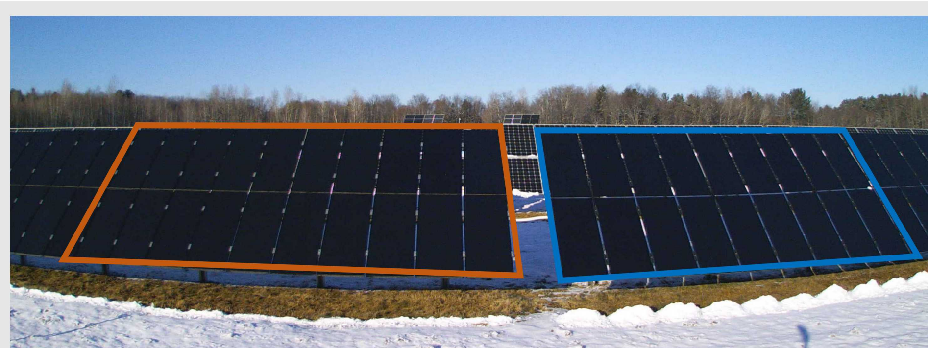
The two PV systems at the VT field site on December 25, 2018. Left modules are framed , right modules are frameless . Highlighted modules are used for snow-coverage analysis.
