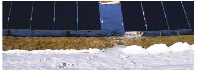
Fig. 7. Snow buildup underneath modules after the December 25, 2018 shedding event. Frameless modules are on the right. Note increased buildup due to faster snow shedding on frameless modules.
