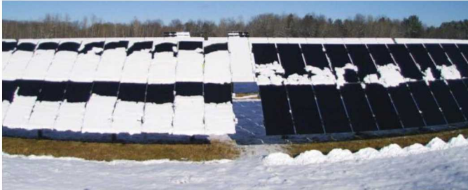
Fig. 3. Framed and frameless PV modules shedding snow at different rates, shown at 10:45 on December 25.
