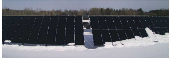
Fig. 8. Increased snow accumulation under the frameless modules on January 30 preventing further sliding.
