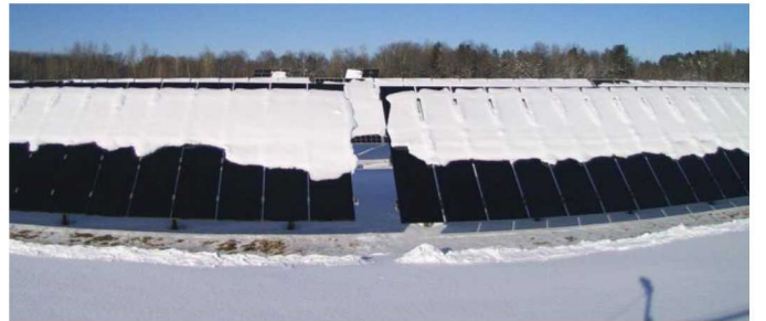
Fig. 5. Framed and frameless PV modules shedding snow at similar rates, shown at 14:15 on January 12, 2019.
