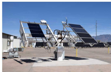
Fig. 1. Eight PV modules tested simultaneously on a two-axis tracker
