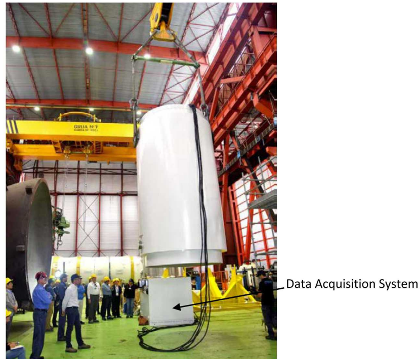
Figure 7. Dry storage cask handling test.
