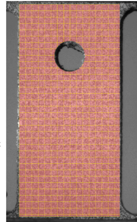
Representative DIC Area of Interest Showing a Grid of 41 pixel x 41 pixel Subsets
