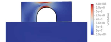
Reconstructed stress field from inverse solution (Sierra-SD)
