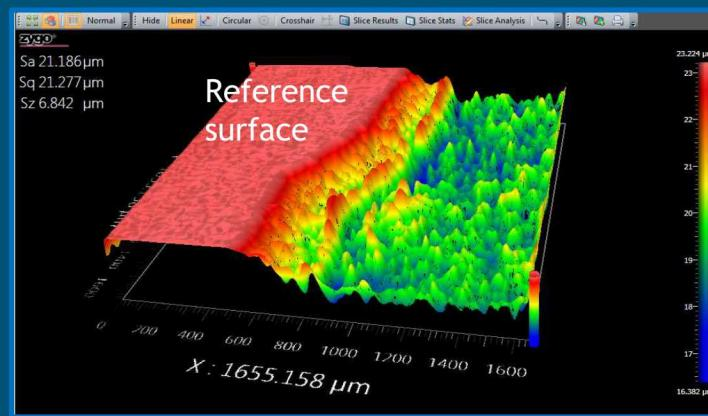
~4.4  $\mu\text{m}$  difference in height can be observed between Reaction and Reference surface
