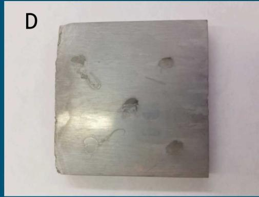
Photographs of post-experiment steel coupons. A. Coupon 113 (SGWB) before cleaning. B. Coupon 113 after cleaning. C. Coupon D (SGWB + NaHS) before cleaning. D. Coupon D after cleaning.
