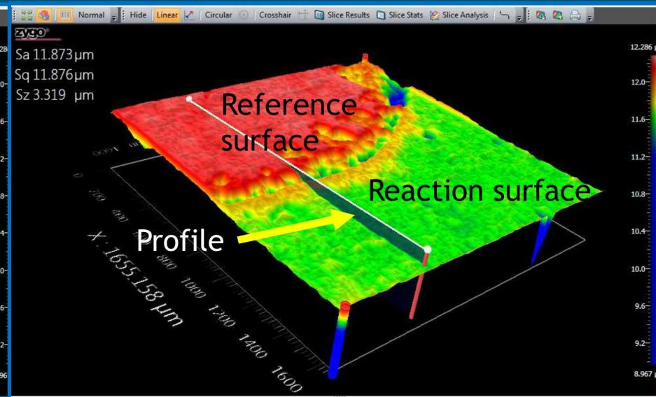
~0.61  $\mu\text{m}$  difference in height can be observed.
