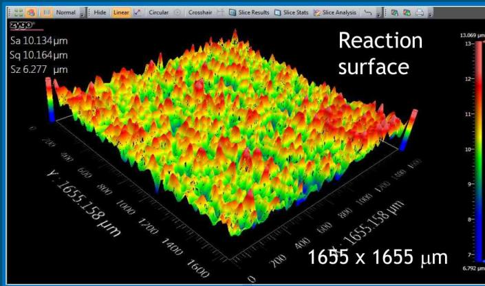
Reaction surface showing an increase in surface roughness
