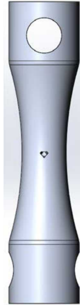
2 mm Through-hole Corner Cube Void
