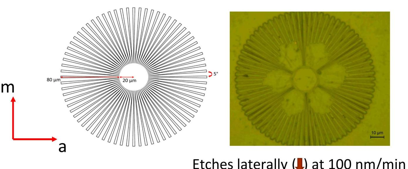
Etches laterally (red arrow) at 100 nm/min vs measured distance of wedge retraction at 6.7  $\mu$ m/min
