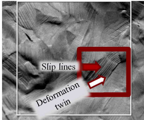
ECC map at final loading increment after significant plastic strain
