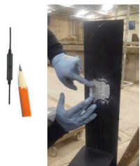
Fiber Bragg Grating for real time strain measurements
