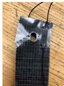
Sub-scale element: bearing stress specimen
