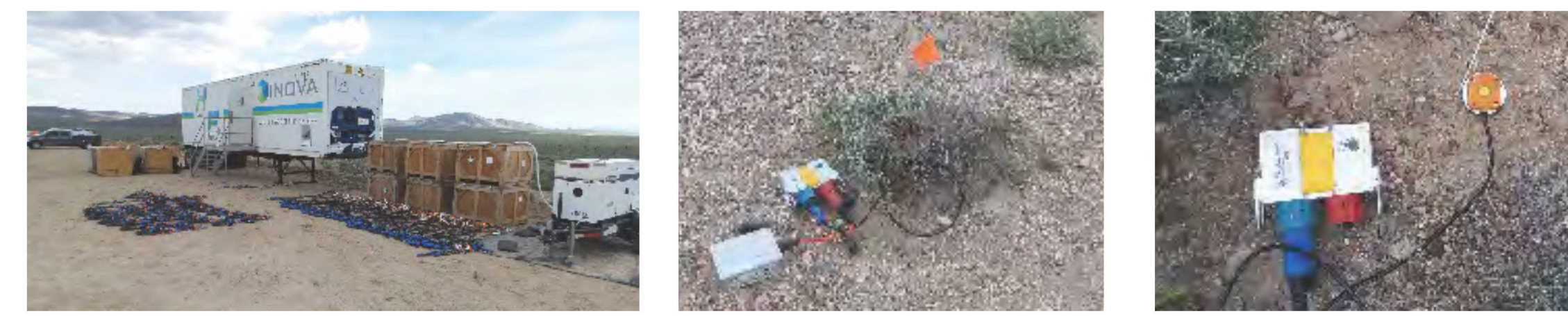
Figure 4. Images of the equipment and truck containing field computer (left), a view of the nodal unit (battery, digitizer/disk, and geophone)(middle), and the emplaced geophone.
