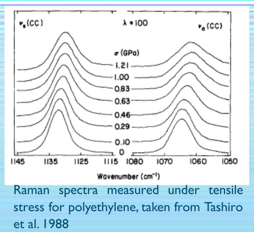
Raman spectra measured under tensile stress for polyethylene, taken from Tashiro et al. 1988
