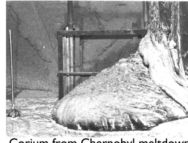
Modeling solidifying systems is a challenge for numerical methods since liquids and solids coexist, interact, and transform into each other during the same simulation. Predicting the spread of corium, for example, in a nuclear reactor accident is difficult since the solid crust that forms severely impacts the flow of liquid beneath.
