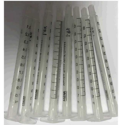
Syringe molded Sylgard specimens
