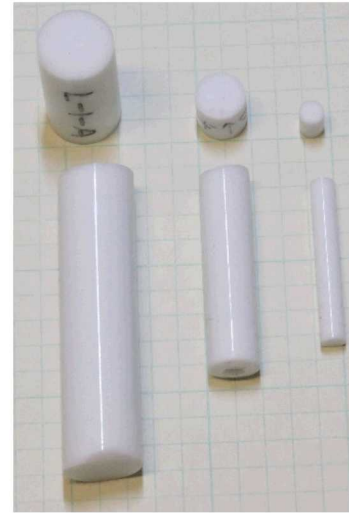
Syringe molded Sylgard specimens
