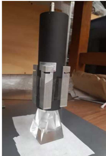
Figure 4. PMT sitting on a custom acrylic light guide [3]
