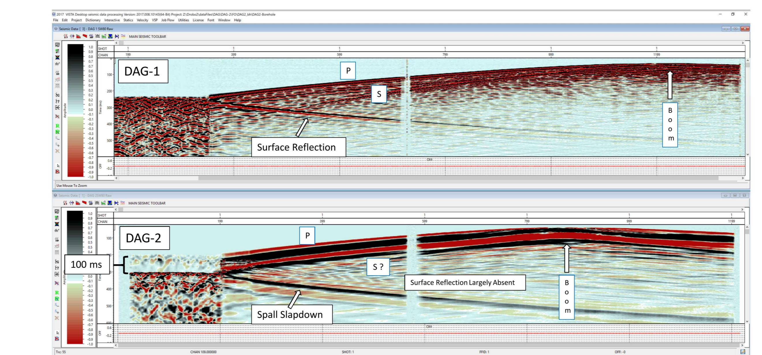
DAG-1 and DAG-2 Recording in hole SW80. Deeper portions of the hole is to the right. The abrupt change in character to ground surface where the fiber transitions to laying on the surface. Notice the immediate reflection from the surface for DAG-1 which delayed 100 milliseconds for DAG-2. We interpret this to be related to surface spall.
