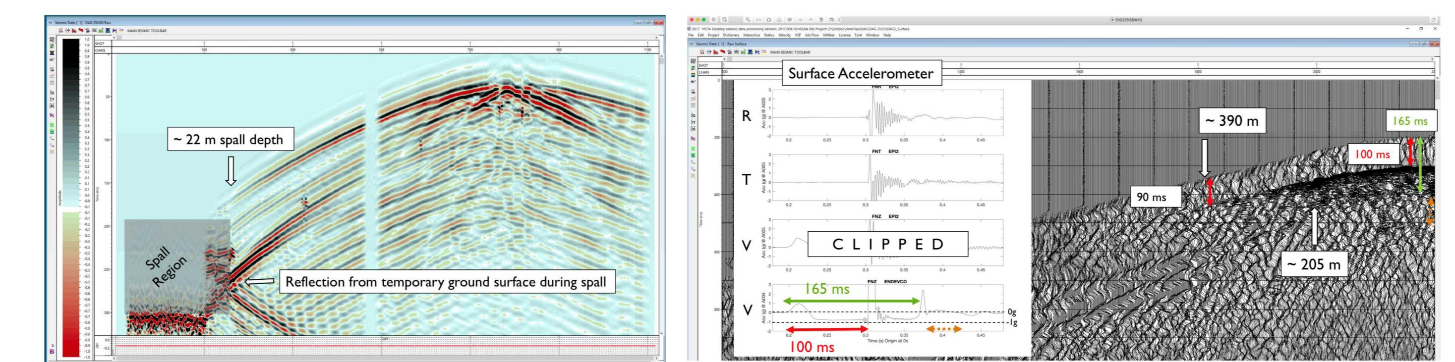
Downhole and Surface Fibers Constrain Both Depth and Width of Spall Zone:
