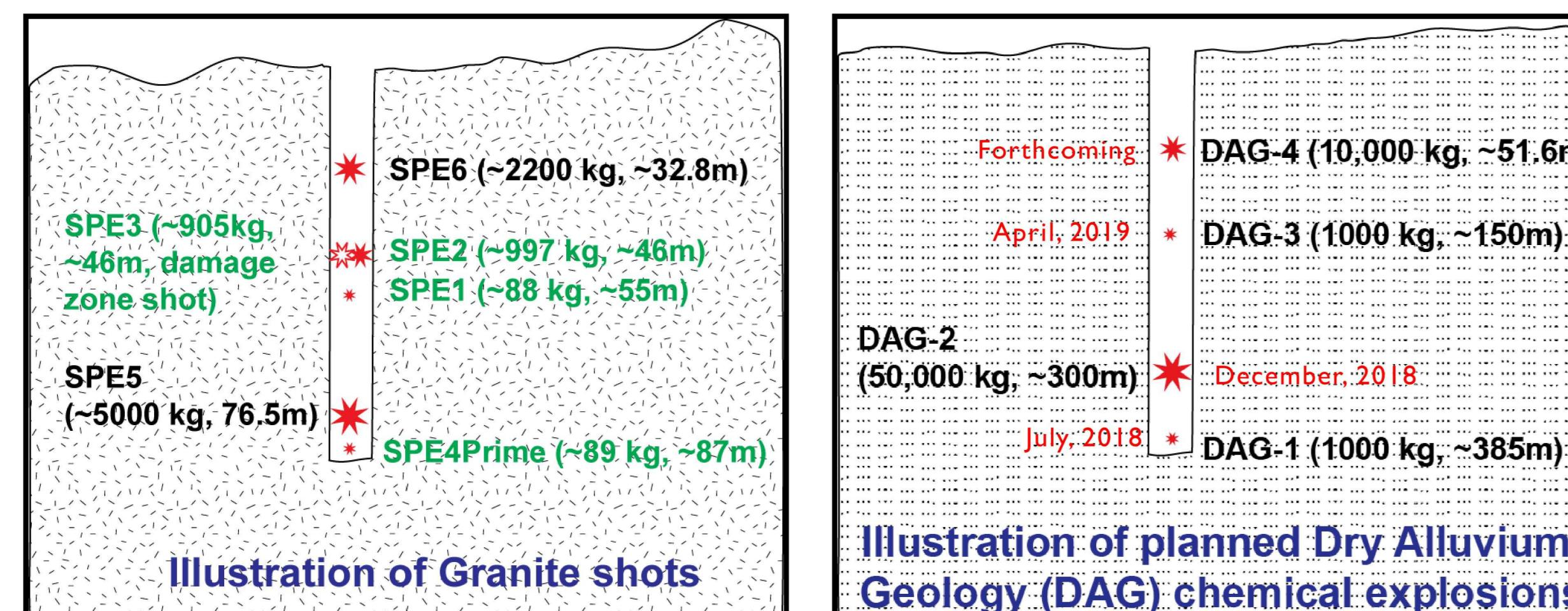
Two dissimilar geologies (granite and alluvium) have hosted the two phases of the Source Physics Experiment. The fiber optic data presented here are for the first two explosions in alluvium. No DAS data was acquired in granite.
