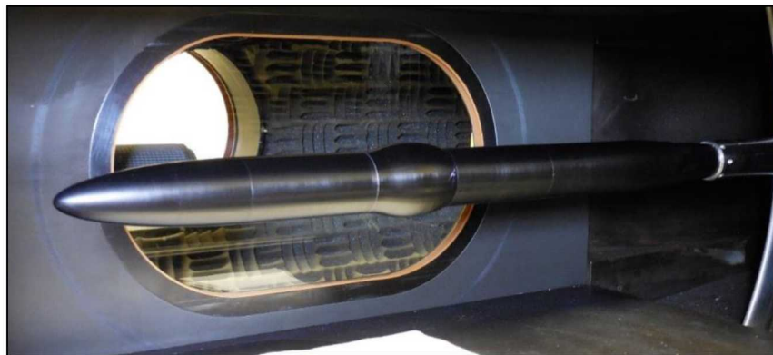
Figure 5. Photo of model in Sandia Trisonic Wind Tunnel.
