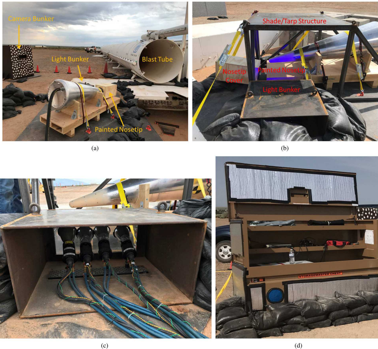
Fig. 1 Blast tube test setup. (a) Overall view of blast tube; (b) System with shade structure and nosetip cover; (c) UV light setup; (d) Job box.
