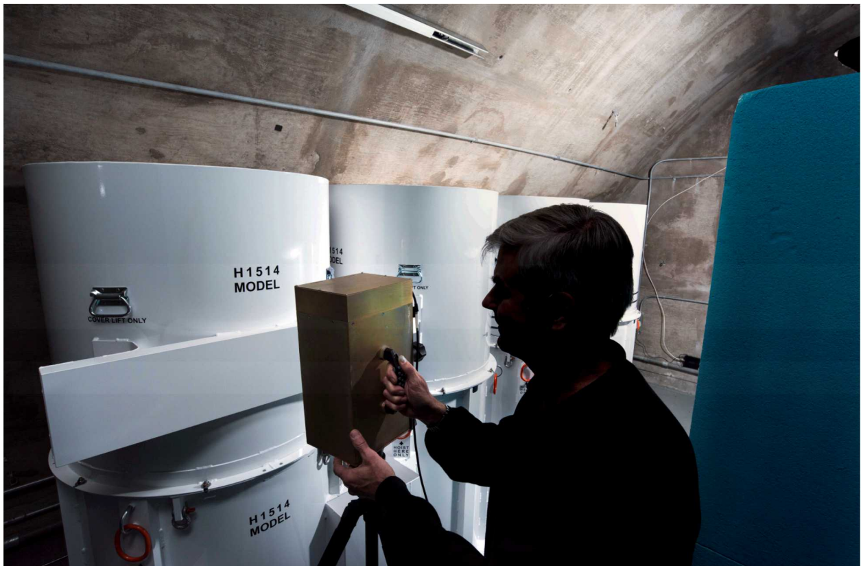
Figure 1 - Radiation Detection Equipment Developed for New START Absence Verification Measurements
