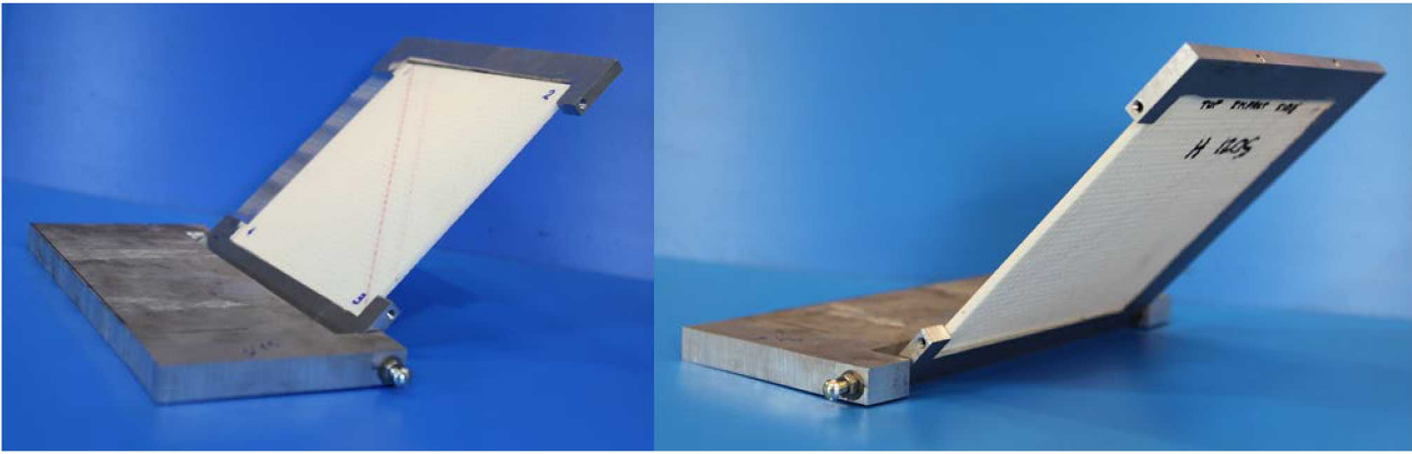
Figure 3. Ballistic testing experimental test fixture. Setup shown is for impact obliquity of 22.5 degrees.
