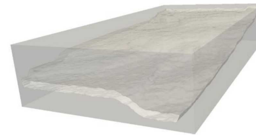
STL image of the fracture without proppants
