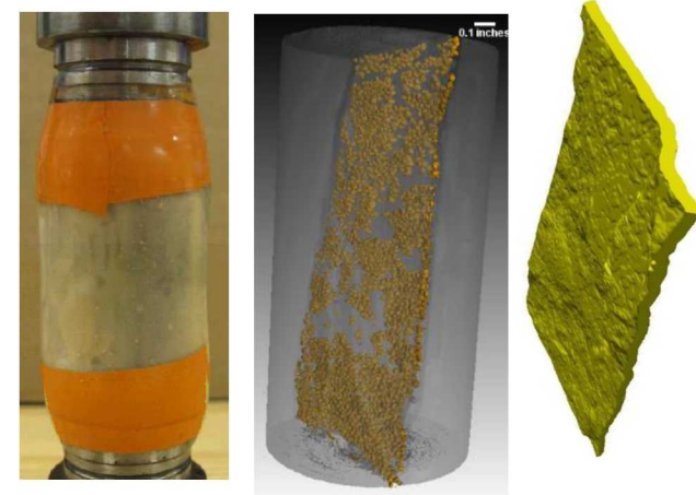
Testing core, rendered image of core, and single fracture network
