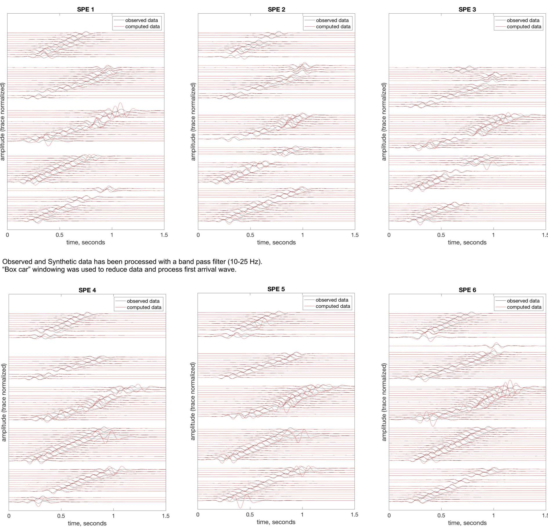
Green's Functions are simulated with the linear orthorhombic algorithm using a point moment tensor source at the source depth. All receivers are used simultaneously in the inversion. A massively parallel implementation of a 3-D seismic waveform simulation algorithm, with the capability to handle fully anisotropic media, was used to generate the Green's functions. This code, *Parahombi*, was developed at Sandia National Laboratories (Preston, 2018).
