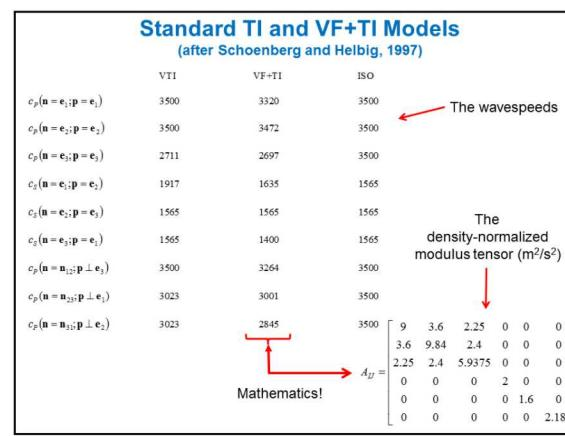
Our initial test modeling utilizes the "standard model" of vertical fractures + transverse isotropic (TI) elastic model of Schoenberg and Helbig (1997), plus its TI and isotropic counterparts.
