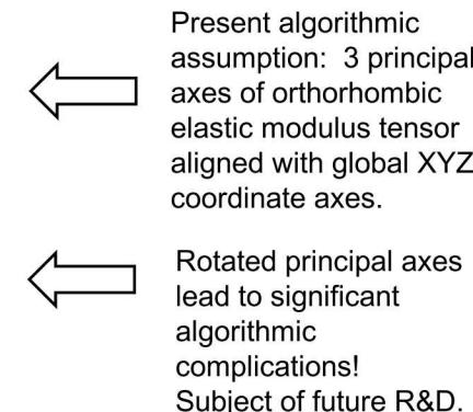
Mathematically, the elastic stress-strain constitutive relations for an orthorhombic body contain nine independent moduli. In turn, these moduli can be determined by observing (or prescribing) nine independent P-wave and S-wave phase speeds along different directions (Brown, 1989):
